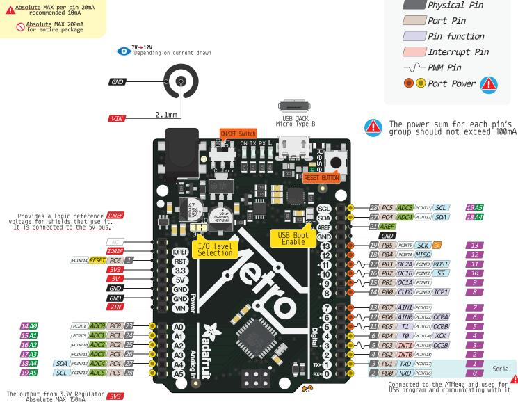
The input voltage to the board when it is running from external power.
